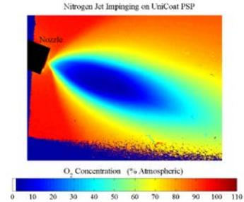
Visualization of a Nitrogen Jet Impinging on a surface painted with UniCoat. The result shows the local concentration of oxygen on the surface.
